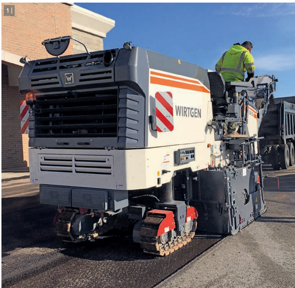
Milling Drum Milling width: 1,800 mm Milling depth: 0 - 330 mm Tool spacing: 18 mm
