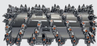
Milling Drum Milling width: 1,800 mm Milling depth: 0 - 330 mm Tool spacing: 18 mm
